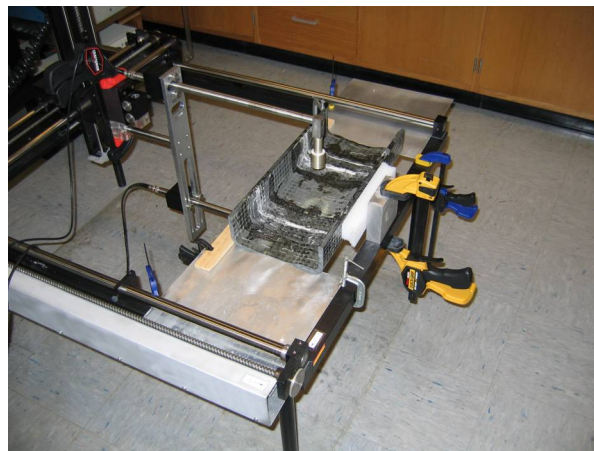
Figure 5.14 The scanning setup used for the CS1 wing spar section.
